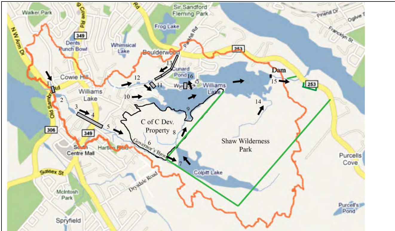
Figure 2. Water flow in the Williams Lake Watershed. Key sources of water supply to Williams Lake with the direction of water flow indicated with arrows. Water courses directed through culverts/underground pipes are indicated with grey rectangles. The boundary of the Williams Lake watershed is shown in red (mapping data courtesy of Dr. Patricia Manuel) and indicates the land where precipitation would normally be fed towards Williams Lake through streams and other water bodies and by percolating through the ground. The lands owned by the Church of Christ Development Corporation (C of C Dev. Property) and the Shaw Wilderness Park are outlined (black and green lines, respectively). Sites referred to in the text of the report are numbered on the map.
