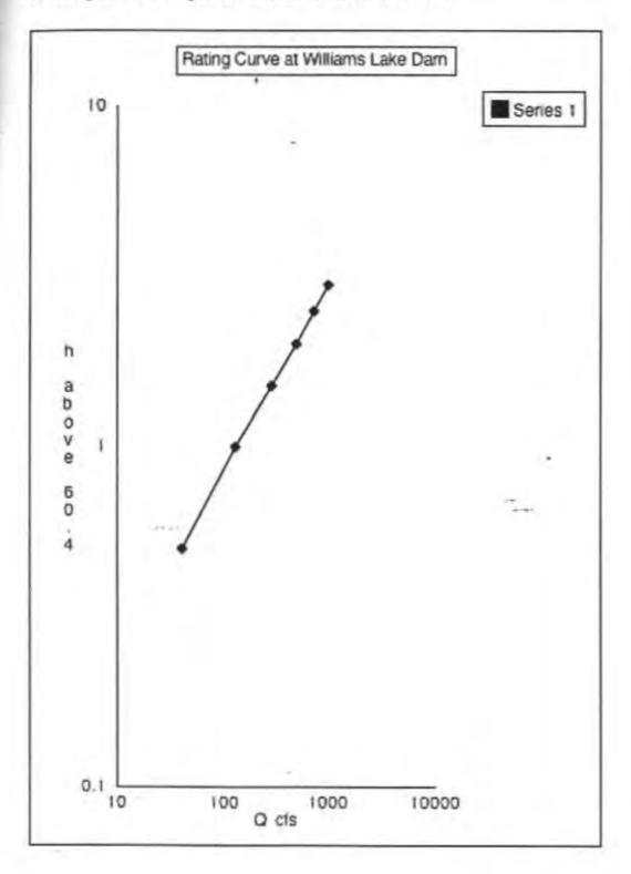
This rating curve was calculated incrementally, assuming the same cross section through the dam/embankment, but adding the contribution of each rise in stage to the flow, using the formula:
